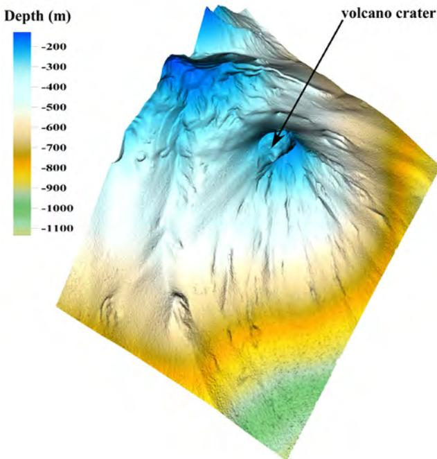
**Figure 3: 5 m lateral resolution digital terrain model (DTM) of the Kick-'em-Jenny (KeJ) current edifice obtained from multibeam data collected during the November 2013 NA039 E/V Nautilus Cruise at KeJ (OET-URI-SRC).**
